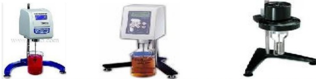
(A) Haake Viscotester VT6L/R (B) Rotational viscometer VISCO BASIC (C) Analog model of viscometer Brookfield BDRV
